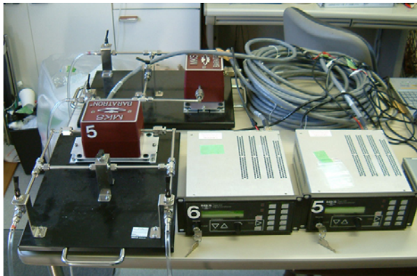
Fig. 6. Pressure gauge for control of airflow rate.
